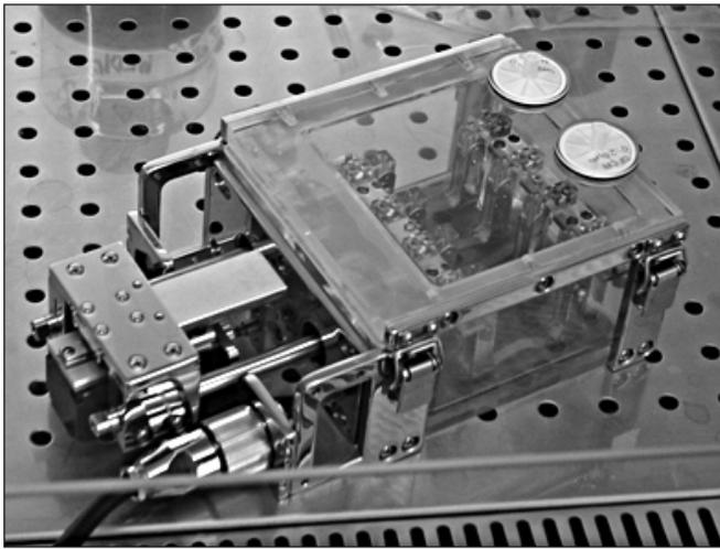
**Fig. 1** - The bioreactor culture chamber with a mechanical stimulation system. The Plexiglas® culture chamber, that houses four biological constructs holding them by means of a system of symmetrical grips, and the stepping motor are housed in the incubator, while the PLC is positioned outside the incubator. For a detailed description see (16).
