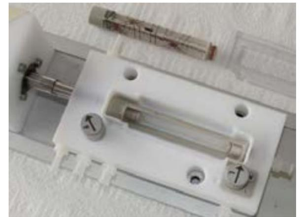
Clinically proven and published tubular constructs bioreactor for hollow organs used in successful human transplantation of bronchus. MiniBreath is a rotating, double-chamber, bioreactor designed for cell seeding and culturing on both surfaces of a tubular matrix and includes rotational movement of the scaffold around its longitudinal axis. Small animal chamber and motor drive controller.
