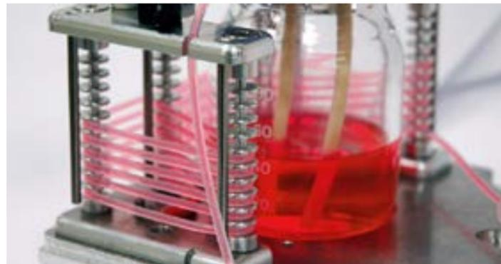
Oxygenator for cell culture systems, equipped with oxygen permeable platinum cured silicone tubing and Luer connectors.
