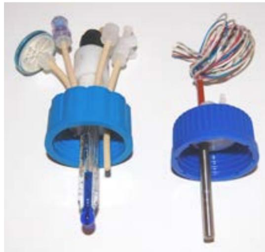
Standard caps (GL45, GL25, etc) with customized inserts to host threaded connectors, special fittings, sensors, probes, heaters, filters and sample ports.
