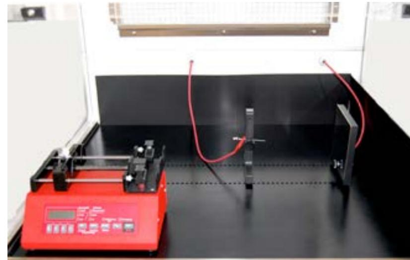
E-fiber is a fully-customisable electrospinning platform consisting of injection stages and application-specific collectors (static or movable), for the laboratory-scale manufacturing of polymeric-nanofibrous matrices.
