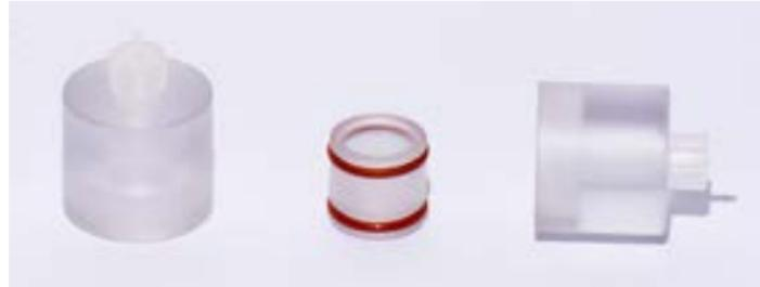
Ergonomic culture chamber for a confined perfusion of cylindrical scaffolds of different sizes.
