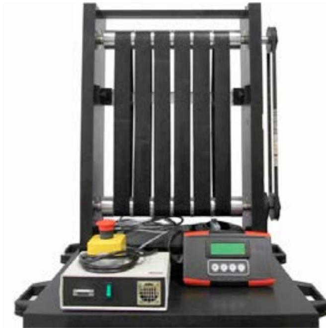
*System for coating a single fiber of nanofibers*
