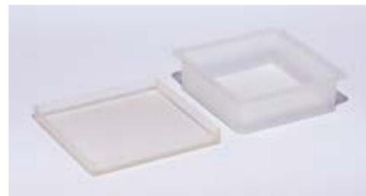
Gas-permeable transparent silicone culture chamber ensures the oxygenation and pH balancing of the culture medium. The silicone chamber is designed with rounded edges in order to avoid stagnation points and has no inlets, breaks, fissures, gaps or holes which could be targets for microbial contamination. Completely autoclavable.
