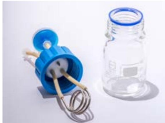
It allows to heat the culture medium that flows through a coil submerged in hot water. Could work inside a cell incubator or with the optional external thermostatic bath, that heat the medium up to 37° C. Useful when you feed your culture with fresh medium stored at 4°C.
