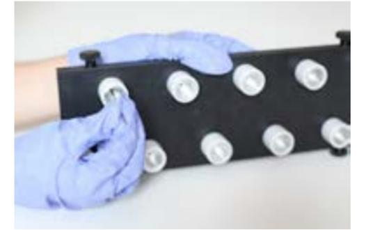
Insulating support to house up to a maximum of 12 spinnerets, used for large planar formats or continuous strip electrospinning machines. Multi-channel syringe pump needed.
