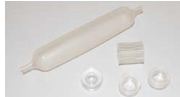
Biocompatible silicone chambers permeable to gases (to allow medium oxygenation in perfect sterile condition).
