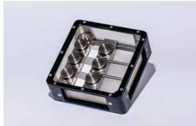
Gym is an incubator-compatible, actuator-driven mechanical stretching bioreactor, which cyclically stimulate up to three tissue engineered constructs in parallel, with a defined displacement stretching pattern.
