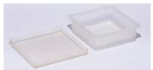
Gas-permeable transparent silicone lid ensures the oxygenation and pH balancing of the culture medium. The silicone lid is designed with rounded edges in order to avoid stagnation points and has no inlets, breaks, fissures, gaps or holes which could be targets for microbial contamination. Completely autoclavable.
