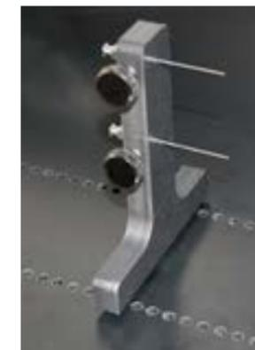
Spinneret support, entirely made of insulating material, with hooks for distance adjusting on the insulating base and insulated screws. 2 spinneret included.
