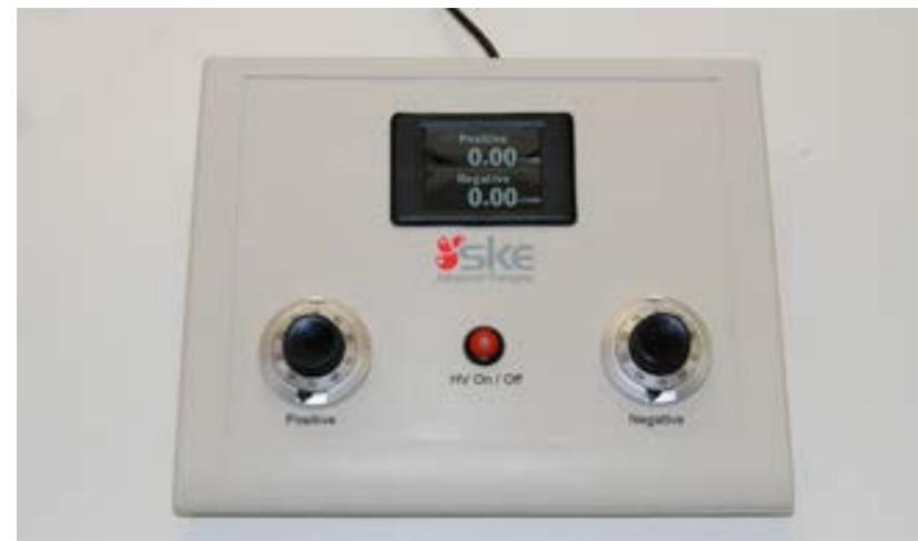
E-fiber is a fully-customisable electrospinning platform consisting of injection stages and application-specific collectors (static or movable), for the laboratory-scale manufacturing of polymeric-nanofibrous matrices.
