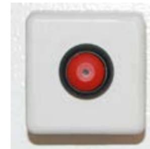
Control pedal or push button for the remote activation of the syringe pump's ON OFF function, useful outside hoods with lowered glass panel.
