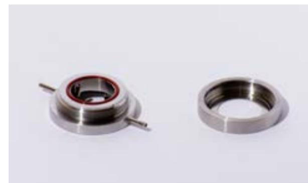
Coverslip holder designed for viewing live cell specimens on upright or inverted microscopes. customer requirements.
