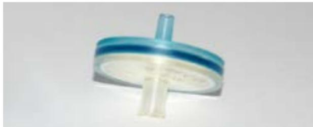
Highest protein retention of all membranes and good binding matrix for macromolecules. Provide fast flow rates with aqueous solutions.
