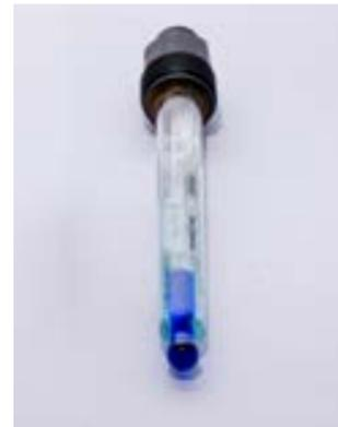
Autoclavable amperometric pH sensor replacement for AutoFeed system.
